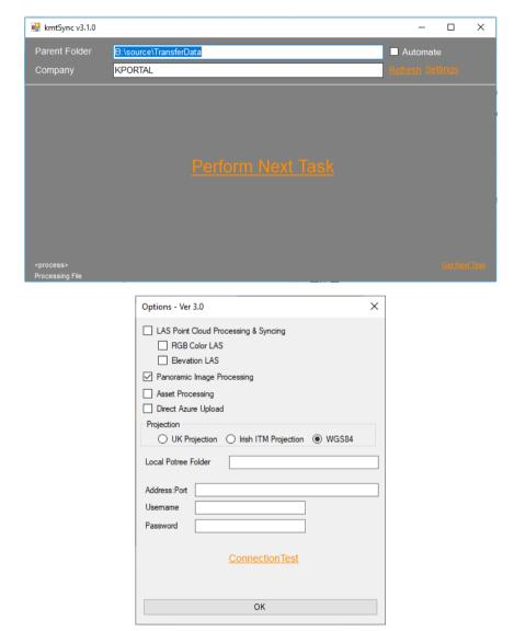
After confirming Connection ensure the setting are correctly configured. For the NCTech camera, this simply requires the Panoramic Image Processing tick box and appropriate Projection – NOTE WGS84 projection will work worldwide
